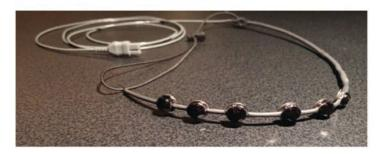
Below the electrode-skin connection is the scalp, forehead muscles, skull and a container filled with cerebrospinal fluid in which floats the brain. All are electrically conductive. An electrical signal from brain neural impulse activity travels through the conductive layers to the surface of the skin.
