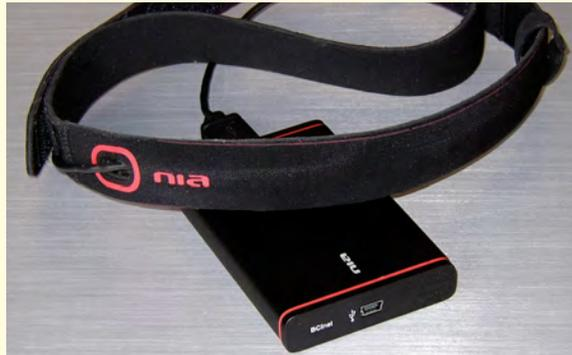
**Figure 2** | The Neural Impulse Actuator: A low-cost combination EEG, EMG, and EOG device
